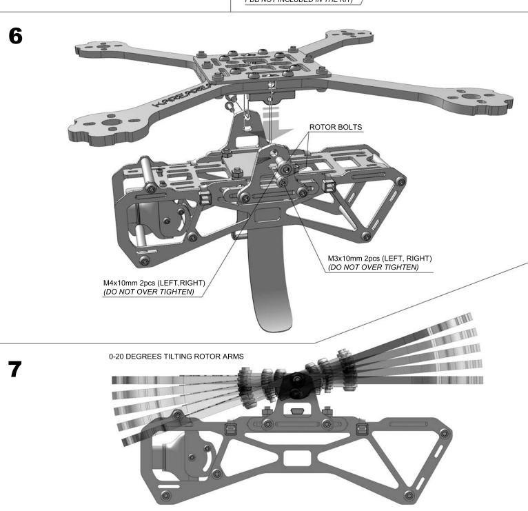
(ONCE YOU HAVE FOUND YOUR OPTIMUM ANGLE FOR THE TILTING ROTOR ARMS, USE LOCTITE TO SEAL AND RETAIN THE ROTOR BOLTS).
